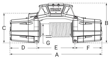
A. 615.9mm C. 199.0mm E. 254.0mm G. 80.0mm B. 266.8mm D. 180.6mm F. 181.3mm Mounting bolt pattern: 254.0mm x 114.3mm
